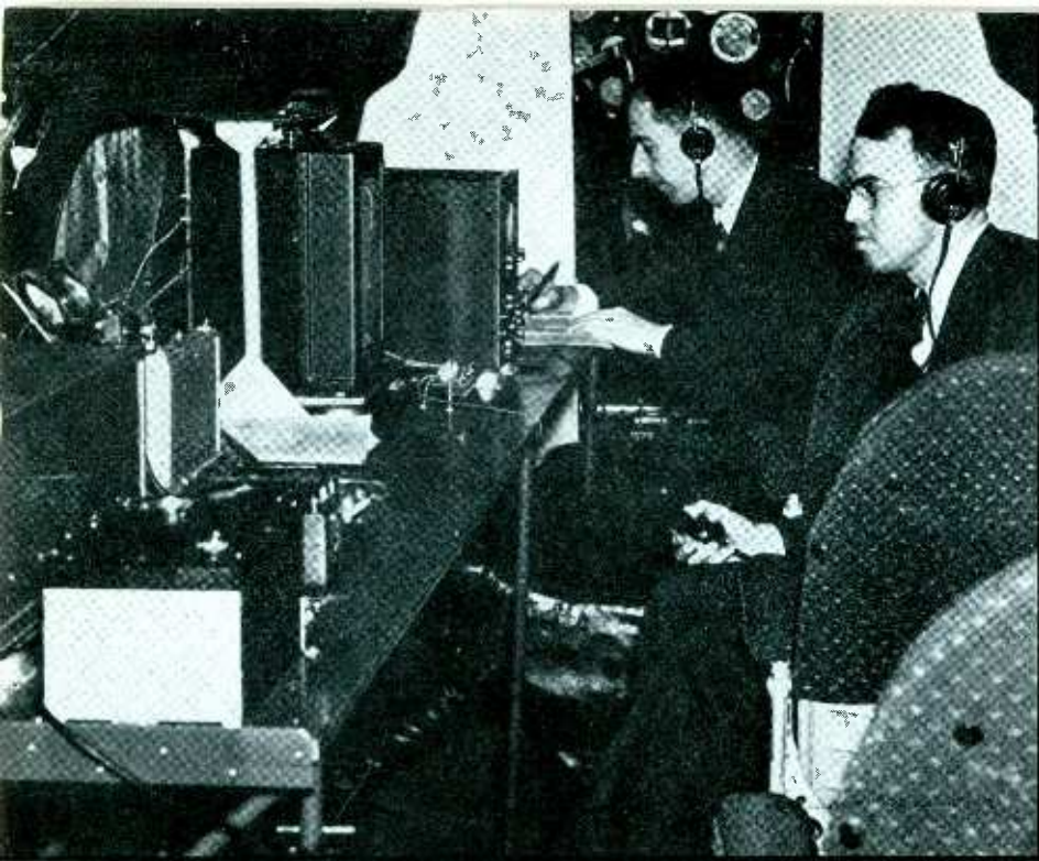
Snow-static studies are carried out in this flying laboratory of the United Airlines. On the bench are automatic recorders for correlating static levels with weather conditions
