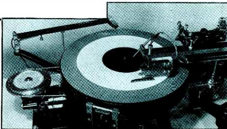
Turntable, recording stylus, and record upon which a black stroboscopic pattern is traced for checking wobble of turntables
