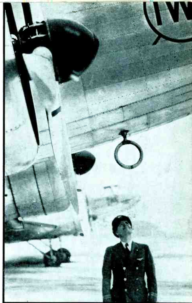
The shielded loop, now required equipment on all transport planes, reduces snow-static by allowing only the magnetic component of the incoming wave to affect the receiver. Note the insulation segment at the bottom of the loop housing
